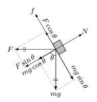
Thus, the block is stationary if  $\theta = 45^{\circ}$ . When  $\theta > 45^{\circ}$ , the force  $F_d > 0$ , and hence the block has a tendency to move down. Thus, the frictional force f acts on the block upwards i.e., towards Q.
