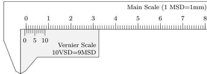
Figure 5: Vernier calipers with negative zero error
