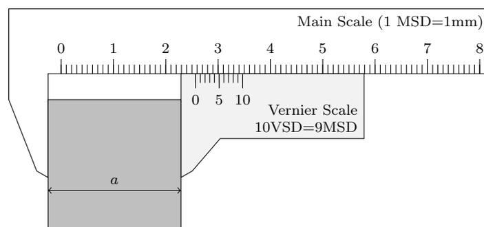
Figure 4: Measuring the edge of a cube
