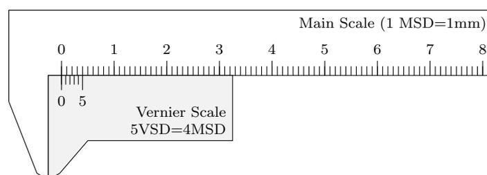
Figure 7: Least Count of a Vernier callipers
