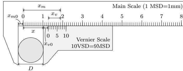
Figure 2: Measuring Diameter of a Marble Ball
