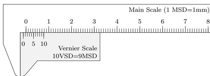
Figure 9: Zero error of the Vernier calipers
