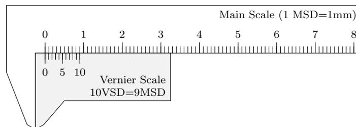
Figure 1: Vernier calipers with no zero error
