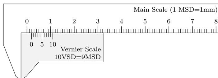
Figure 8: Zero error of the Vernier calipers
