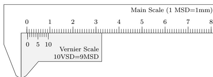
Figure 3: Vernier calipers with positive zero error
