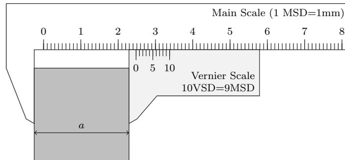
Figure 6: Measuring edge length of a cube
