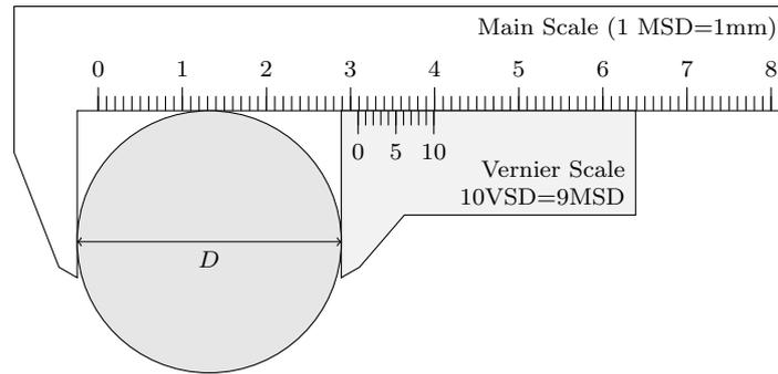
Figure 11: Measuring diameter of a sphere with an erroneous Vernier calipers
